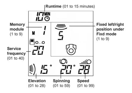
(a) LCD Display under MANUAL FIXED MODE
