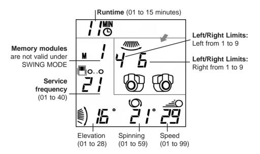
• Button function under MANUAL SWING MODE. (Because the operation of most buttons is identical to the MANUAL FIXED MODE, please refer to the previous explanations about the same buttons. Following are the explanations about the unique buttons under the MANUAL SWING MODE that are different from the MANUAL FIXED MODE).
