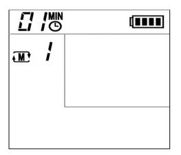
(b) LCD Display under MEMORY/CYCLE MODE with modified settings (the memory module is 2 and the setting is modified (not empty)).
